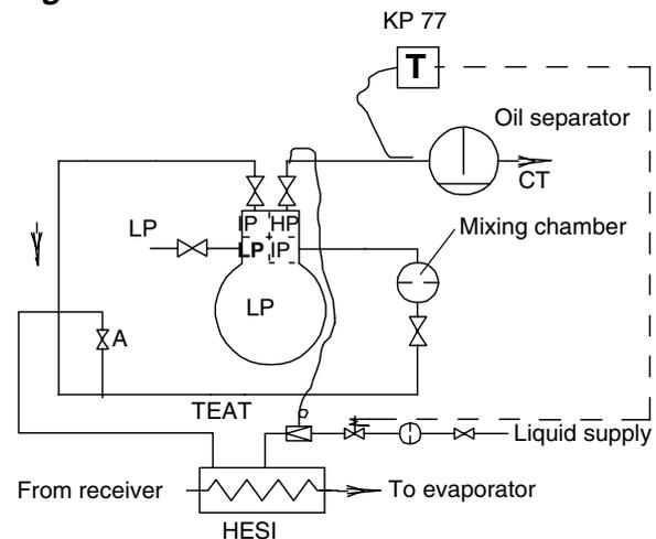
The sensor of the TEAT valve is placed in a sensor pocket at the HP discharge branch of the compressor, and a proper thermal contact is obtained by means of the heat conducting compound. The solenoid valve is opened by the KP77 thermostat whenever the temperature of the pressure pipe exceeds 55°C [131°F].
