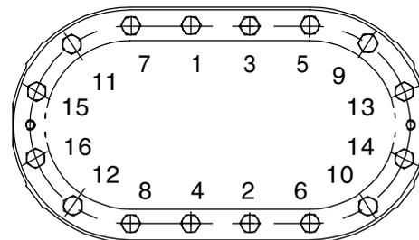
Once the top cover has been fitted, remove the **long plug** and insert the **short plug**. The top covers must be mounted as shown in the following chart.
