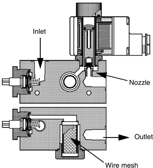
From the stop valve the oil passes a wire mesh, which can be removed and cleaned. The filtered oil now passes the solenoid valve, which must be **closed** at dead coil whenever the compressor is stopped. When the compressor is operating, the
