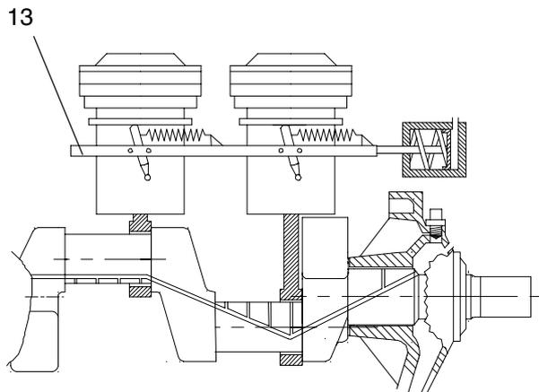
The capacity regulating system including the frame, pos. 13, is activated by the compressor oil pressure and controlled by means of solenoid valves fitted on the compressor. At a capacity reduction two suction valves are forced open at a time. In this case no compression takes place in the relevant cylinders as the sucked in gas in the cylinders is pressed back to the suction chamber through the suction valves.
