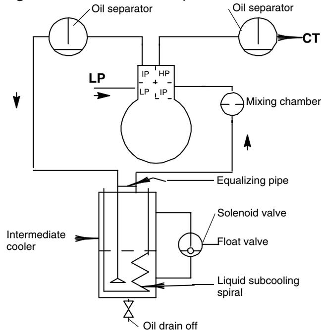
In the liquid subcooling spiral the refrigerant flowing from the receiver to the evaporator in the refrigeration plant is cooled. The intermediate cooler is dimensioned so that the cooled gas is free of liquid refrigerant before leaving the top of the intermediate cooler. It is important to check that the float valve is operating correctly and keeping the liquid level constant. Frosting of the liquid level pipe on the intermediate cooler indicates the liquid level.
