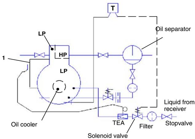
The filter filters off any dirt particles in the liquid. The filter element can be removed and cleaned. The stop valve can block the cooling system from the refrigeration plant.
