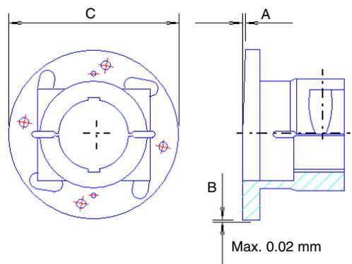
Alignment must be kept within the values stated in Table 6.6.
