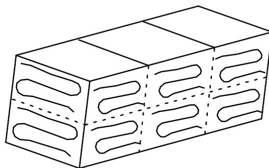
The **measuring grid** is divided into **fields of max.1 sq. m** each. The measuring is carried out by moving the sound level meter in a kind of back and forth movement, as illustrated in Fig. 6.44. The sound level meter now calculates the total sound power level  $L_W$  for the entire unit.
