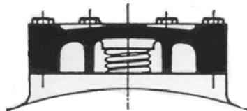
**Fig. 4.60** Air-cooled Side Cover
