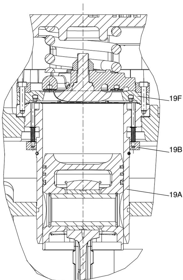
The unloading ring, pos. 19B, is activated by two rocker arms, pos. 15A, Fig. 4.41, one at each side of the cylinder liner. The rocker arms, which are placed in ball sockets, pos. 15B, are moved back and forth by the unloading frame, pos. 13.
