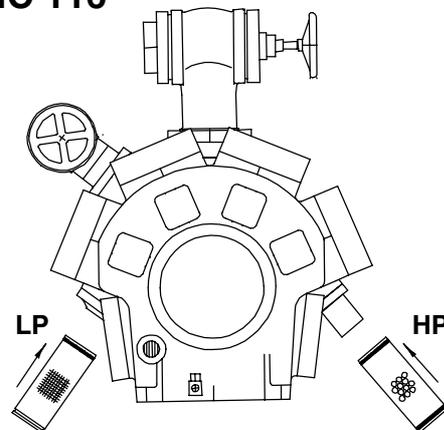
The suction filter fitted on the righthand side opposite the high-pressure cylinders has a closed end-bottom which must face upwards and close towards the suction stop valve. This suction filter must be fitted with O-rings at both ends.
