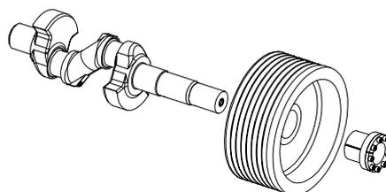
When dismantling the belt pulley, loosen the screws on the clamping unit.
