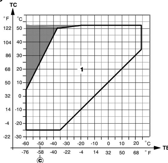
By using the table which is situated next to the oil recommendation diagram, select the recommended code number and thus the recommended oil. In the example above there are thus 3 possibilities: PAO3, AP1 or M1. However, M1 is only recommended for moderately loaded compressors.
