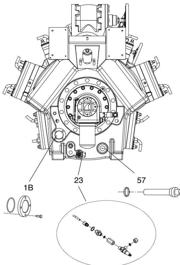
**Oil draining valve**, pos. 23, for draining and charging of oil. An inner socket at the draining valve ensures that the oil sump is properly drained so that the compressor does not have to be opened when changing oil and filters.
