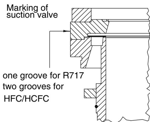
The cylinder lining and suction valve form an integral unit which can be dismantled by removing the screws 19N.
