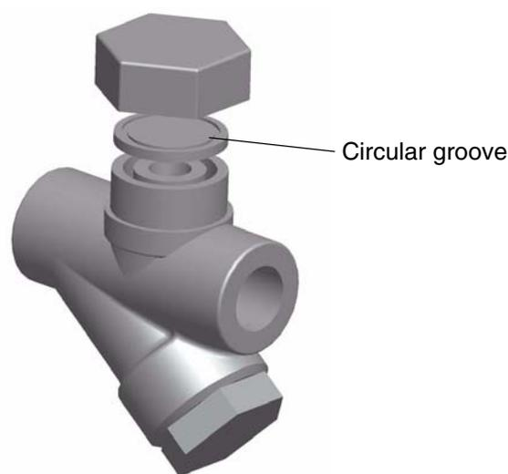
Correct fit with circular groove upwards and radial scratch down towards seats.
