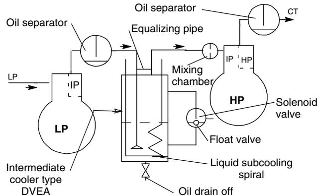
Fig. 4.55 TSMC 100 Compressor
