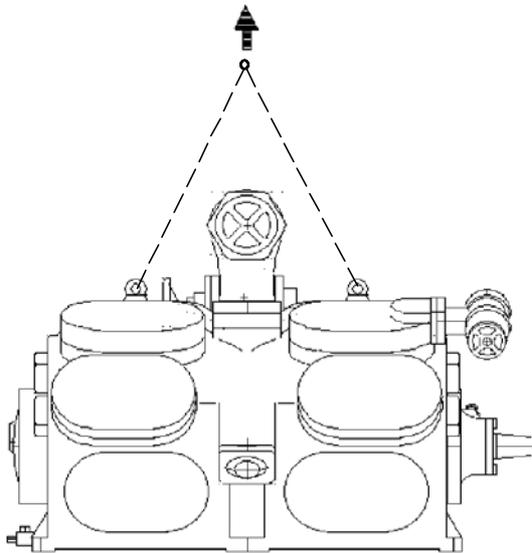
The unit is lifted in the lifting eyes, which are welded onto the base frame and clearly marked with red paint. When the unit is lifted, make sure that
