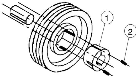
When **dismounting** the belt pulley, first dismount the two or three screws, pos. 2, and then mount one or two of the screws in the free hole/s where there is only a thread in the side which **faces** the bushing. By tightening the two screws evenly, it is now possible to press the belt pulley off the bushing. The bushing and the belt pulley can now be dismounted manually.
