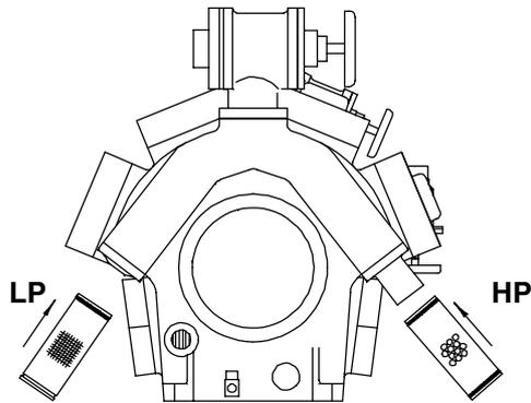
**On TSMC compressors**, the suction filter located on the lefthand side opposite the low-pressure cylinders (see drawing) is the same type as on SMC compressors, i.e. open at both ends and with an O-ring in the end facing up towards the suction stop valve.
