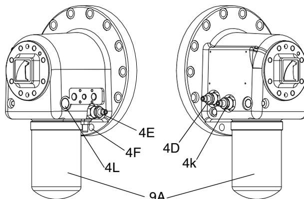
**Differential pressure monitoring** of the oil filter is carried out using a differential pressure switch mounted directly on the pump housing as standard. The signal serves as a warning to indicate that the filter must be changed. The filter has extra capacity in order to avoid using the signal for an alarm which forces the compressor to stop.
