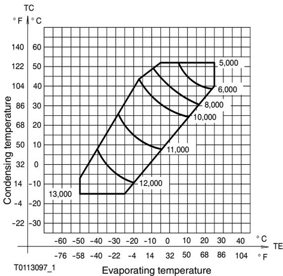
**Fig. 11.2 HCFC/HFC/R290 - SMC 100 S-L**
