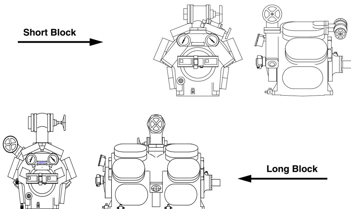
Single-stage compressors are designated **SMC** which is an abbreviation of **SABROE Multi-cylinder Compressor**. As for the two-stage compressors the letter **T** has been added to indicate **Two** stages.
