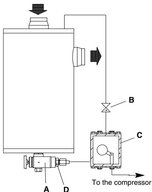
The separated oil is drained through stop valves A and filter D to the float vessel C, and here the float valve opens at an increasing oil level and returns the oil to the crankcase.
