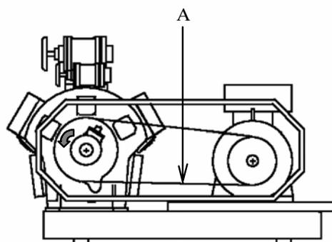
The compressor pulley is bored with a cylindrical hole and is fitted to the crankshaft with a clamping unit. The end of the crankshaft and the outer face of the clamping unit must be aligned. Thus the belt pulley can be mounted on the crankshaft without previous adjustment. It must be tightened with the nine screws on the clamping unit, see fig. 6.41. The screws are tightened with a torque wrench.
