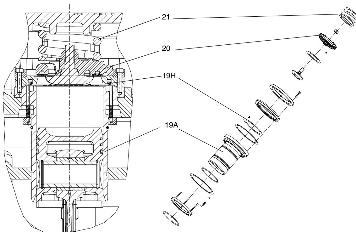
The pistons, pos. 18, are made of aluminium with two hard-plated piston rings and one oil scraping
