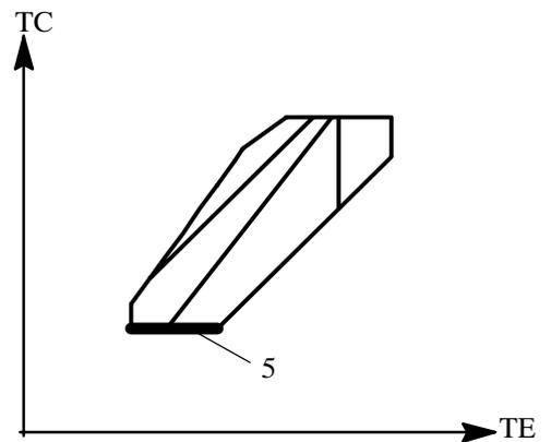
**6. Minimum Difference between Condensing and Evaporating Temperature:**
