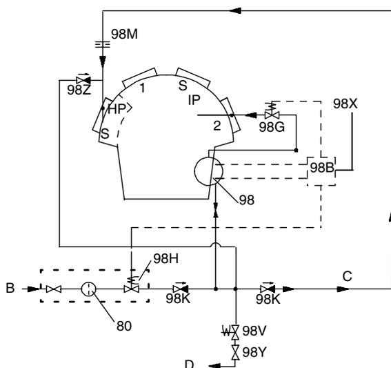
Filling and evacuation of the pump vessel is controlled by two level sensors, pos. 98C, Fig. 4.71. By means of the control box, pos. 98B, the sensors control the solenoid valves, pos. 98G and pos. 98H, so that they open and close simultaneously.
