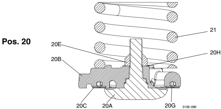
As shown in the above drawing, the function of the discharge valve Pos. 20 is partly to allow the compressed gas to pass from the compression chamber of the cylinder to the discharge chamber beneath the top covers and partly to create a seal from the discharge chamber to the cylinder.
