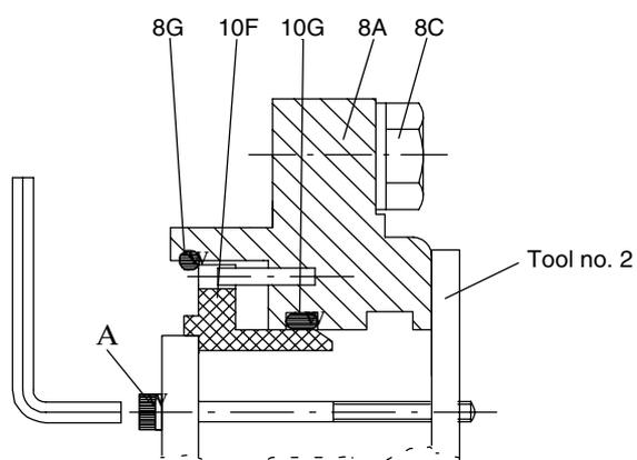
9. Dismantle slide ring 10E by turning the four Allen screws 10J max. 2-3 turns; the entire unit can then be taken out with the fingers or by using two screwdrivers inserted into the external groove on the slide ring Pos. 10E and moved in the direction of the arrow as illustrated in Fig. 13.15.
