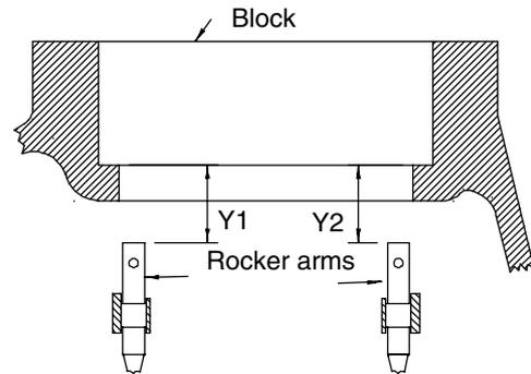
2. The rocker arms must be in their vertical position i.e. with the short screw pos. 12D and gasket 12E fitted. The measured distances "Y1 and Y2" may not vary more than max. 0.25mm.
