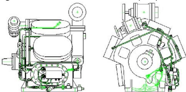
The thermo pump is mounted as a side cover on the compressor and works by pressing the refrigerant into the canal system on the top covers and into the oil cooler which - depending on the operating conditions - is built into the crankcase.
