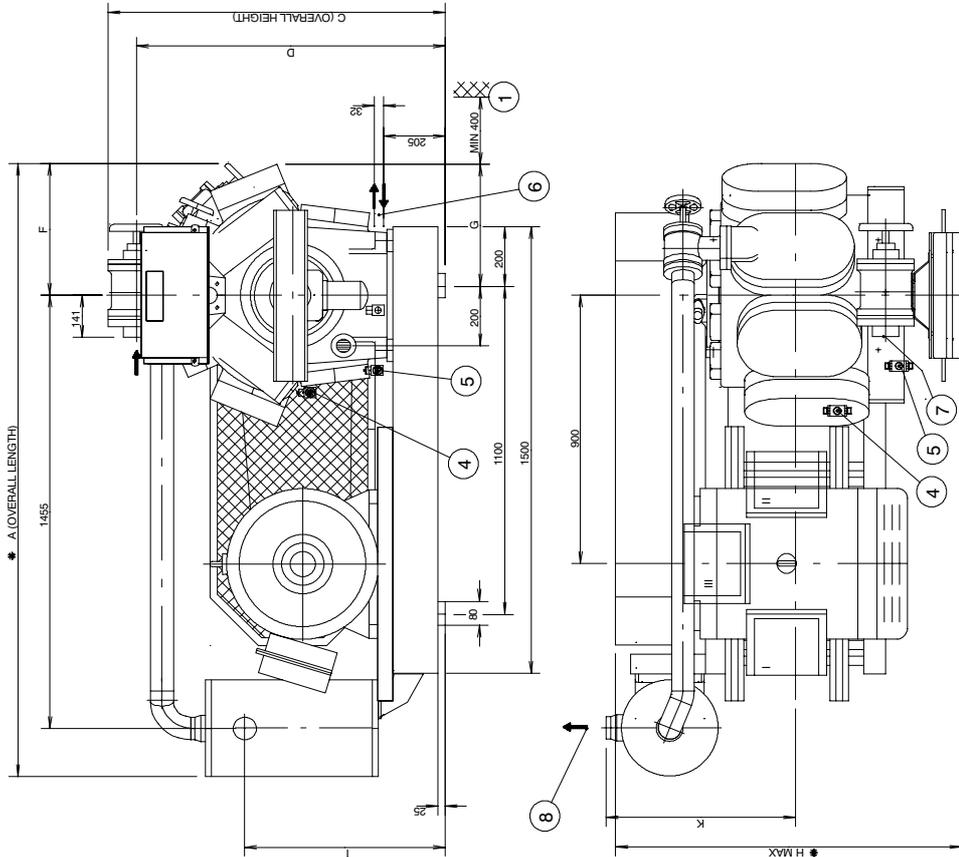
\* OVERALL LENGTH AND WIDTH VARIES ACCORDING TO MAKE OF MOTOR AND TYPE FOR EXACT LENGTH USE DIMENSION H IN TABLE
