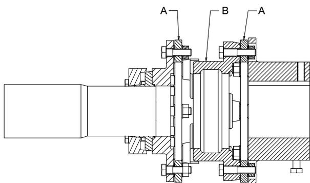
With the torsionally resistant coupling the oscillatory weight of the rotor in the electric motor works as a "flywheel", providing the compressor with a stable and vibration free operation during all kinds of operating conditions and capacity stages.
