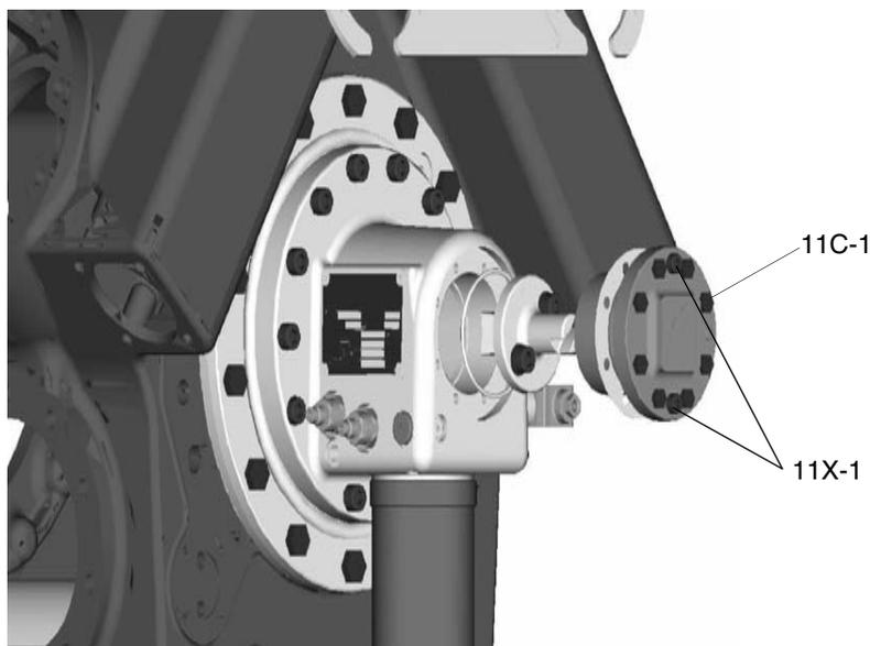
The oil pump is a gear pump which is run by the crankshaft by means of a guide. The oil pump direction of rotation is marked on the cover.
