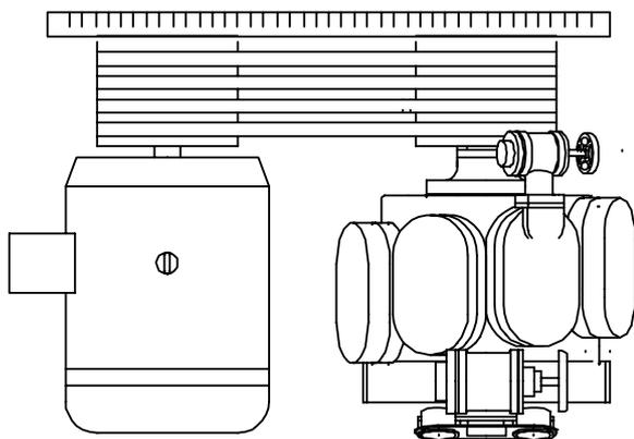
By letting the electro motor drive the compressor through a V-belt drive, the speed of the compressor can be selected so that the max. capacity corresponds to the capacity requirements of the plant.
