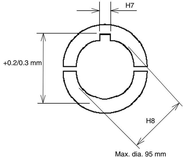
As seen in the above drawing, Fig. 6.31, the coupling hub is slit up axially and clamped to the motor shaft with two screws.
