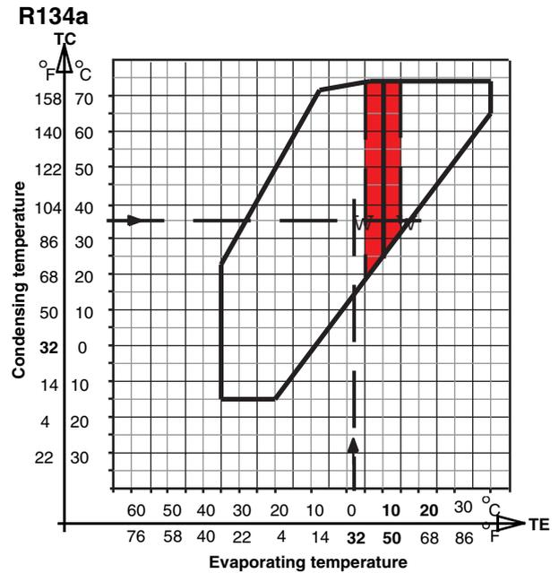
By using the table which is situated next to the oil recommendation diagram, select the recommended code number and thus the recommended oil. In the example above an oil with code number E5 can be used.
