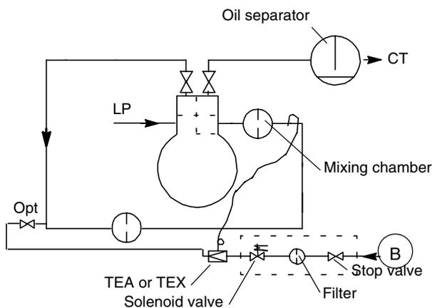
In the system in Fig. 4.56 the liquid refrigerant conveyed to the intermediate pipe is regulated by a **thermostatic expansion valve type TEA (R717) or TEX (R22)** with a sensor placed on the intermediate pipe close to the HP stage.
