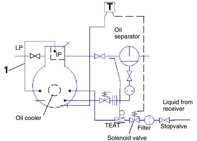
**Fig. 4.63** Two-stage TSMC Compressor R717
