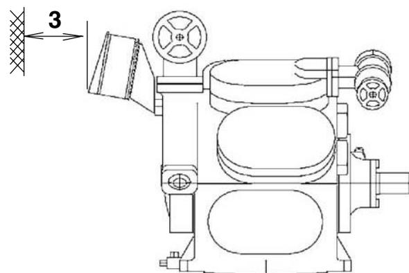
Enough room must be left around the compressor to allow the operating personnel to operate the compressor ① and carry out service work on the compressor ②. Space should be considered ③ as
