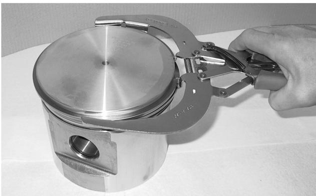
Fig.76: Remove the piston rings and the oil scraper ring (tool not in tool set)
