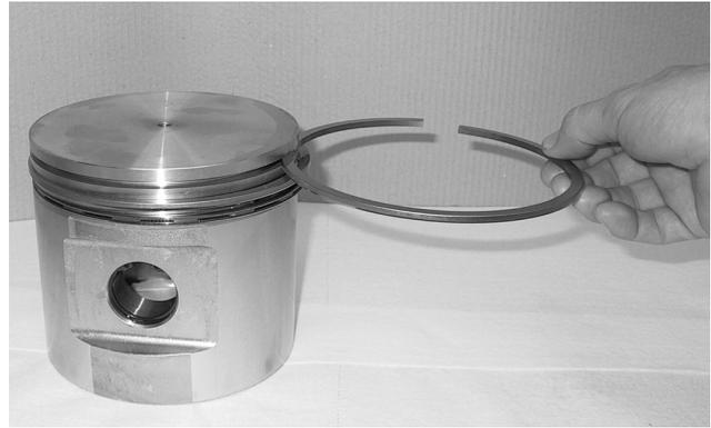
Fig.77: Replace the NEW piston rings; Roll each piston ring and oil scraper ring in the corresponding groove around the piston to trace parts that have become wedged.
