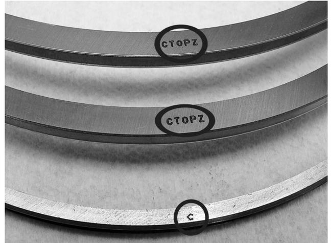
Fig.82: When placing the rings, pay attention to the word "CTOPZ" and "C" on the oil scraper ring
