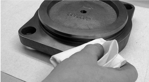
Fig.176: Clean the groove carefully with a clean, non fibrous cloth
