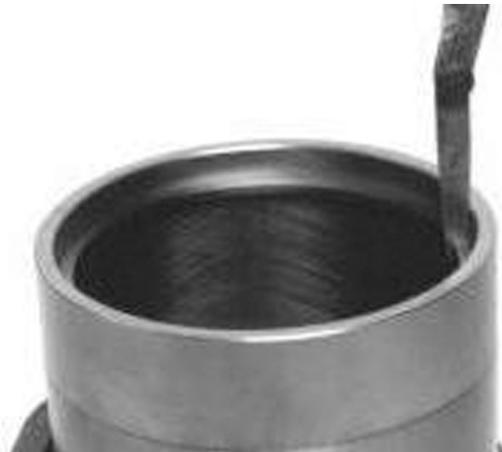
Fig.78: Check the gap in each piston ring by placing it in an unworn part of the cylinder liner. These unworn parts can be found at about 10 mm from the bottom of the cylinder liner. The maximum gap as given ( )
