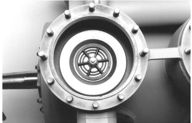
Fig.153: Top view of discharge valve assy
